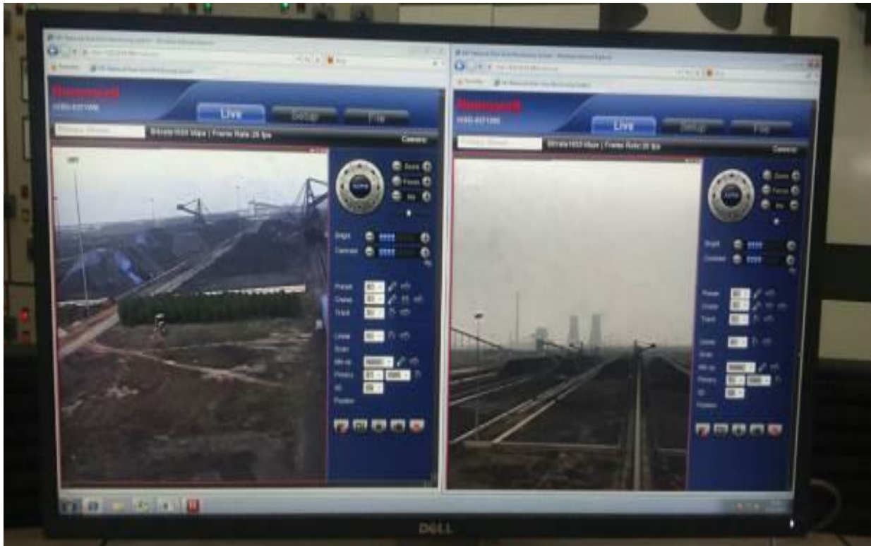
CONTINUOUS MONITORING OF DUST SUPPRESSION SYSTEM AT COAL YARD USING PTZ CAMERAS
